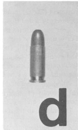
FIG. 2—(a) Colt .25 caliber tear gas pen gun (90% of actual size), (b) components of Colt pen gun (90% of actual size), (c) firing pin (left) and barrel (right) (actual size), and (d) .25 caliber jacketed cartridge (actual size).
